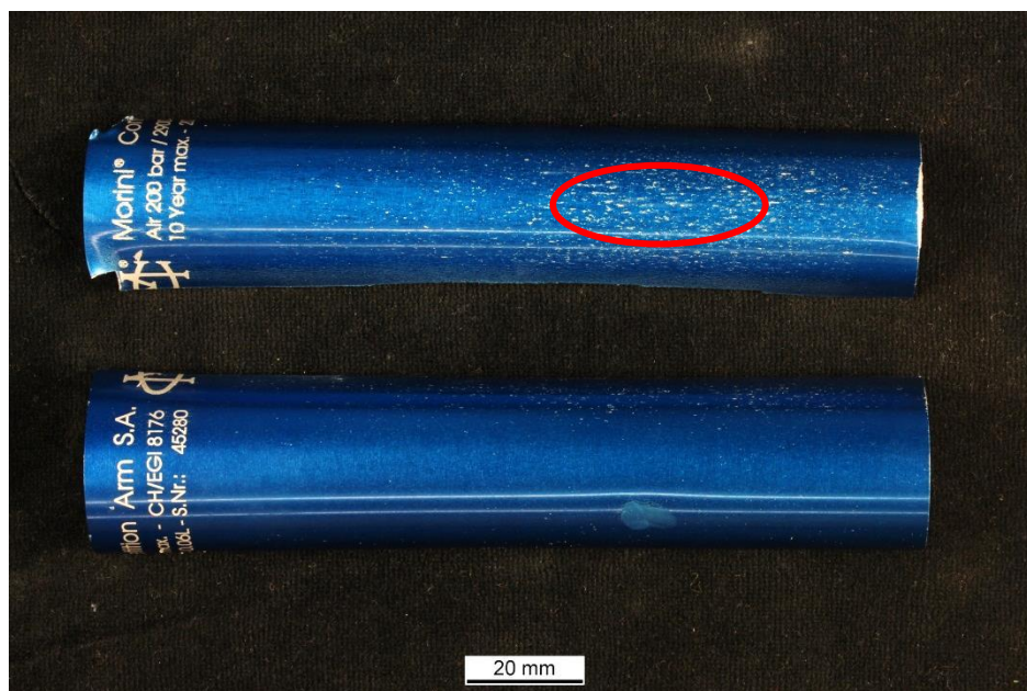
Photo 2: The broken specimen as delivered. The areas of corrosion attack are conspicuous (circle).
