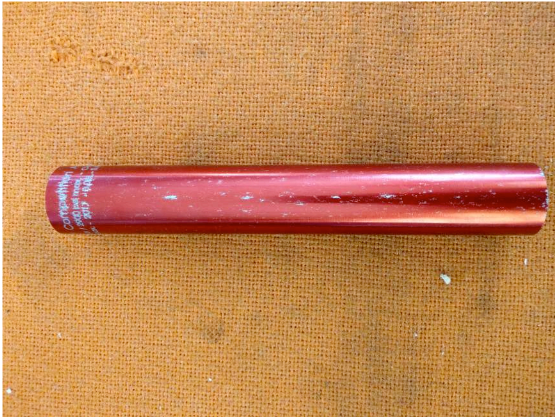
Corroded bottle which cannot be used
